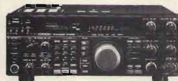
KENWOOD TS 850 S/AT RTX in SSB, CW, AM, FM e FSR - 100 kHz, 30 MHz - 108 dB - 100 W - 100 memorie - presa RS 232 - 2 VFO - Alim. 13,8 V.
